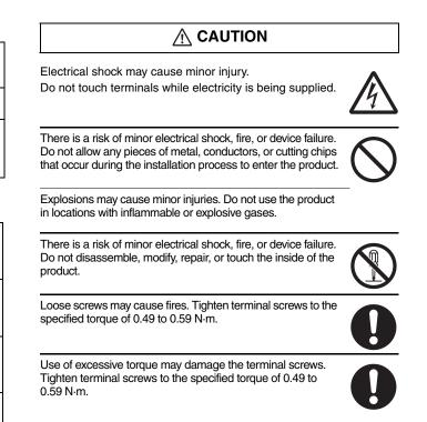
Use of the product beyond its life may result in contact welding or burning. Make sure to consider the actual operating conditions and use the product within its rated load and electrical life count. The life of the output relay varies significantly with the switching capacity and switching conditions.
