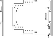
• Removing from the DIN Track Pull down on the bottom hook with a flat-blade screwdriver and lift up on the product.
